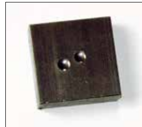
Brinell Test Piece after Brinell Indent
